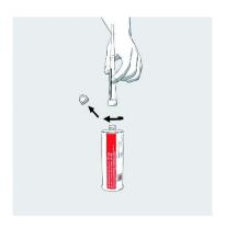
Hold the cartridge vertically with the tip pointing upward, unscrew the sealing cap and screw on the mixer provided.
