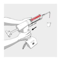
Start pressing out **ZZ**<sup>®</sup> 330 Fire Protection Foam and discard non-uniform initial material.
