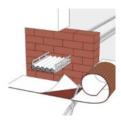
Cut off a sufficiently long piece of **ZZ® 451 Fire Protection Bandage** and after removing dirt from the installation, peel off the protective film and apply the bandage.
